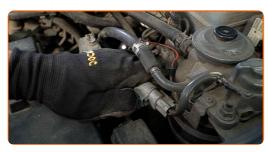
Loosen the fastening clamps of the fuel filter pipes. Use round-nose pliers.
