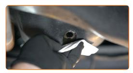
Screw in the new drainage plug and tighten it. Use a combination spanner #14. Use a torque wrench. Tighten it to 25 Nm torque.
