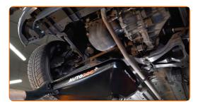
Unscrew the oil filter. Use the 76/14-F socket. 9
