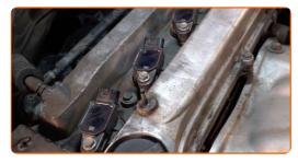
Tighten the fasteners of the ignition coils. Use a drive socket #10. Use a torque wrench. Tighten it to 8 nm torque.
