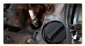
Screw new spark plugs and tighten them. Use the spark plug socket #16. Use a torque wrench. Tighten it to 25 nm torque.
