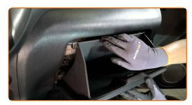
Press on the side walls of the glove box to reinstall the stoppers.
