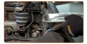
Unscrew the bracket of the water-in-fuel sensor. Use a drive socket #8.
