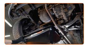
9 Unscrew the oil filter. Use the 76/14-F socket.
