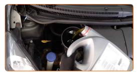
Replacement: engine oil and filter – TOYOTA Corolla VII Estate (E100).
