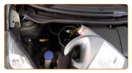
Replacement: engine oil and filter – TOYOTA Corolla VI Liftback (E90).
