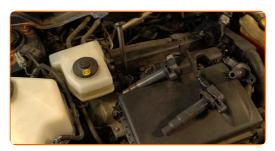
Screw new spark plugs and tighten them. Use the spark plug socket #16. Use a torque wrench. Tighten it to 18 nm torque.
