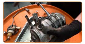
Remove the protective case of the fuel filter.
