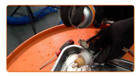
Install the new O-ring of the water-in-fuel sensor.
