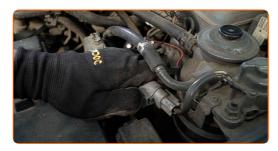
Loosen the fastening clamps of the fuel filter pipes. Use round-nose pliers.
