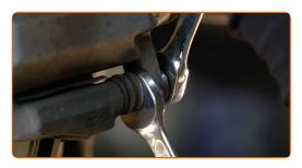
10 Remove the brake caliper.
