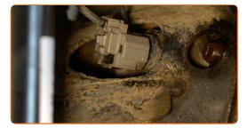
Disconnect the ABS sensor wiring.
