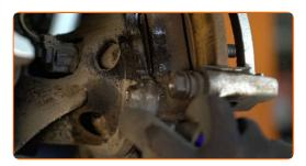
Unscrew the caliper bracket fastening. Use a drive socket #14. Use a tap wrench. Use a ratchet wrench.
