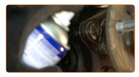
Clean the ABS sensor connector. Use all-purpose cleaning spray.
