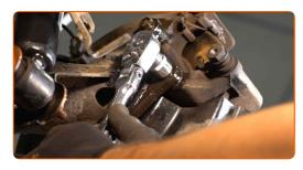
Remove the caliper bracket.
