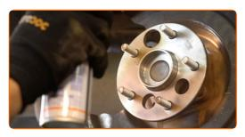
30 Install the brake disc.
