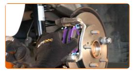
Install the brake caliper and fix it. Use a combination spanner #17. Use a drive socket #14. Use a torque wrench. Tighten it to 35 Nm torque.
