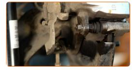
Unscrew the brake caliper fastening. Use a combination spanner #14. Use a combination spanner #17.
