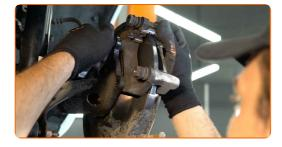
Tighten the brake caliper bracket. Use a drive socket #14. Use a torque wrench. Tighten it to 57 nm torque.
