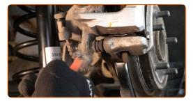
Detach the parking brake cable from the bracket on the brake caliper. Use water pump pliers.
