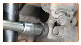
Remove the brake caliper.
