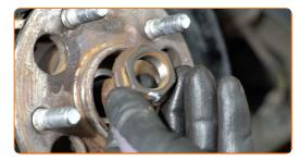
Remove the wheel hub bearing.
