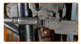
Install the brake caliper retaining spring.
