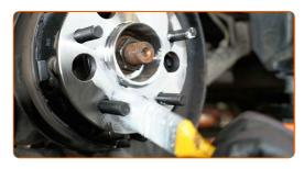
Install the brake disc.
