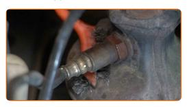
6 Unscrew the oxygen sensor fastener. Use a flare nut spanner #22. Use a ratchet wrench.
