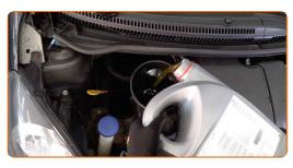
Replacement: engine oil and filter – TOYOTA Corolla Rumion (E150).
