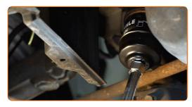
Prepare a container for the old oil filter. Put the old oil filter in the container.
