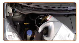
Replacement: engine oil and filter – TOYOTA Corolla IX Hatchback (E120).
