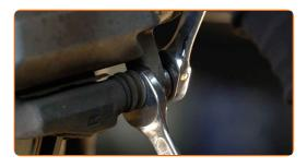
10 Remove the brake caliper.
