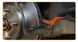
Treat the brake caliper piston. Use a brake cleaner.
