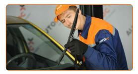
Remove the blade from the wiper arm.
