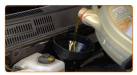
Replacement: engine oil and filter – TOYOTA Corolla Hatchback (\_E7\_). Tip from AUTODOC:
