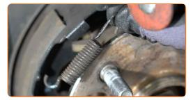
Treat the wheel hub bearing fasteners. Use WD-40 spray.
