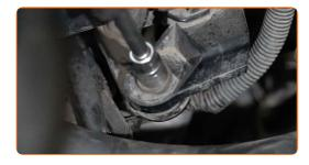
Connect the air intake pipe to the air filter housing.
