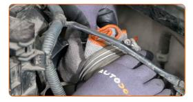
Move the air filter housing aside.
