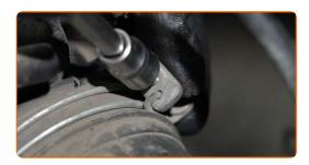
Screw in the fasteners of the air filter housing. Use a drive socket #10. Use a ratchet wrench.
