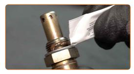
Install the new oxygen sensor.
