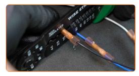
Shrink the heat shrink tubes of the solder sleeves. Use a heat gun.
