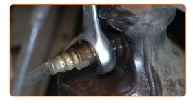
Remove the oxygen sensor.
