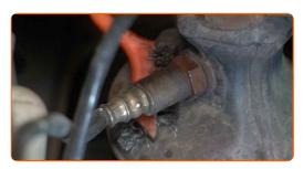
6 Unscrew the oxygen sensor fastener. Use a flare nut spanner #22. Use a ratchet wrench.
