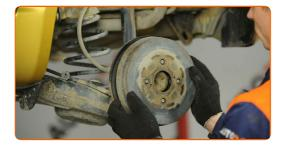
Replacement: brake drum - TOYOTA COROLLA Estate (\_E12J\_, \_E12T\_). Tip:
