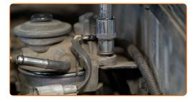
Remove the fuel filter. Put the old filter cartridge in the container.
