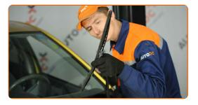
Remove the blade from the wiper arm.
