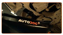
Unscrew the oil filter. Use the 76-14F socket. Use a ratchet wrench.
