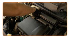
Tighten the oil filler cap.
