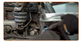
Unscrew the bracket of the water-in-fuel sensor. Use a drive socket #8.
