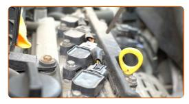
Unscrew the fasteners of the wiring harness bracket. Use a drive socket #10. Use a ratchet wrench.
