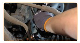
Screw in the sway bar link fasteners. Use a drive socket #14. Use a ratchet wrench.
