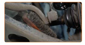
Unscrew the fastener connecting the stabilizer link to the stabilizer bar. Use a drive socket #14. Use a ratchet wrench.
