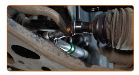
Tighten the fastener connecting the stabilizer link to the shock strut. Use a drive socket #14. Use a torque wrench. Tighten it to 44 Nm torque.
