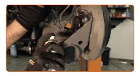
Connect the ABS sensor wiring.
