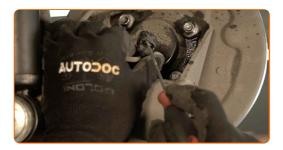
Disconnect the ABS sensor wiring.
