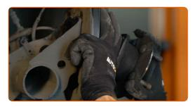
Clean the hub bearing mounting seat. Use a wire brush.
