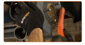
Remove the brake drum.
