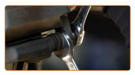
10 Remove the brake caliper.
