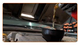
Replacement: engine oil and filter – TOYOTA Celica III Hatchback (A60). Tip from AUTODOC experts:
