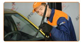
Remove the blade from the wiper arm.
