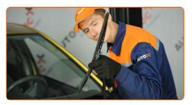
Remove the blade from the wiper arm.
