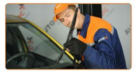
Remove the blade from the wiper arm.
