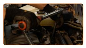
Replacement: spark plugs – TOYOTA CELICA Convertible (ST16\_, AT16\_).
