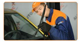
Remove the blade from the wiper arm.
