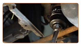
Prepare a container for the old oil filter. Put the old oil filter in the container.
