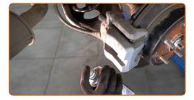
Unscrew the brake caliper fastening. Use a drive socket #14. Use a tap wrench.
