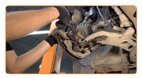
Remove the caliper bracket.
