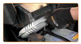
Unscrew the clamp and fasteners on the air filter intake pipe. Use a drive socket #10. Use a ratchet wrench.
