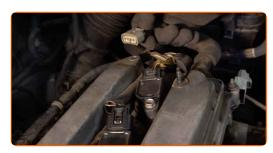
6 Unscrew the ignition coil bracket. Use a drive socket #10.
