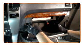
Remove the cabin air filter housing.
