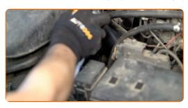
Unscrew the oil filter. Use the 76-14F socket. Use a ratchet wrench.
