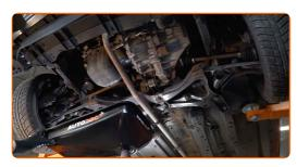
Unscrew the drain plug. Use a drive socket #15. Use a ratchet wrench.
