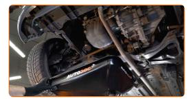
Unscrew the oil filter. Use the 76/14-F socket.
