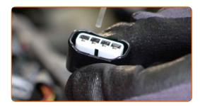
Plug in the connectors of the ignition coils.
