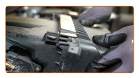
Press the air filter cover clips into place.
