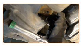
Clean the area of the oil pan drainage hole.
